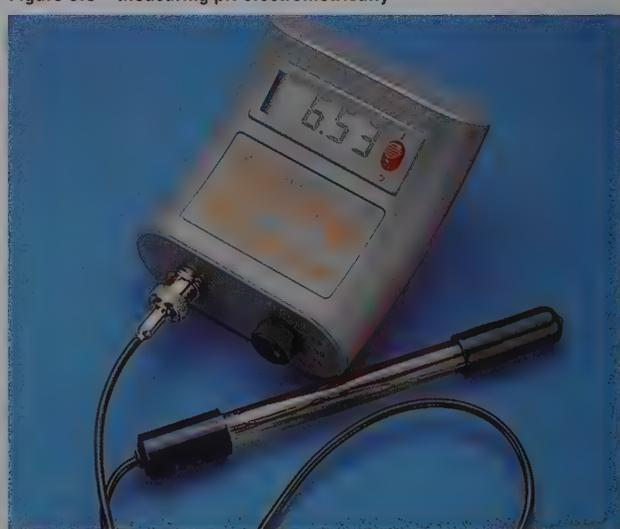
**pH can be measured electrometrically** during fieldwork by using a battery-operated pH meter. This carries a special electrode probe, which is placed in the sample of unknown pH (such as soil or water). The meter measures the potential difference produced in the probe unit; this potential difference is proportional to the hydrogen ion concentration. The electrode is standardised in a buffer solution of known pH just before it is used in the field
