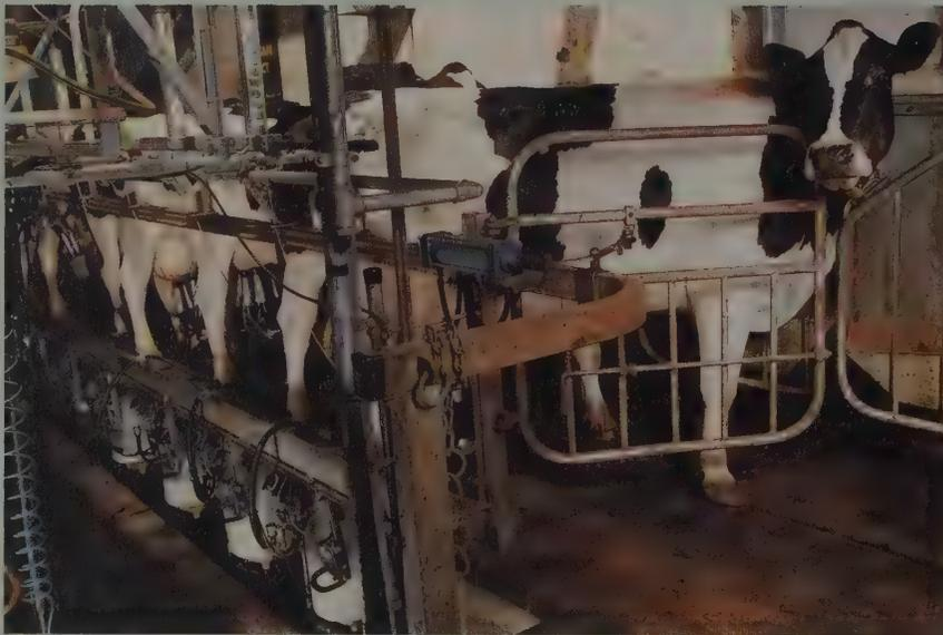
There is a milking machine (set of suction cups that fit over the cow's teats) to each two cows. Milk is withdrawn into storage bottles behind the cows' rear feet (the milk volume can be measured) and then transferred to the bulk tank in the dairy nearby. The clusters can be removed automatically when the flow of milk stops.
